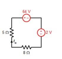
We have transformed the 8 A current source in parallel with the 8  $\Omega$  resistor into a 64 V voltage source in series with the same resistor. The original resistor was changed to an open circuit, and that resistor was then inserted in series with the new voltage source. (We also compressed the circuit.) (8 A)(8 Ω) = 64 V
